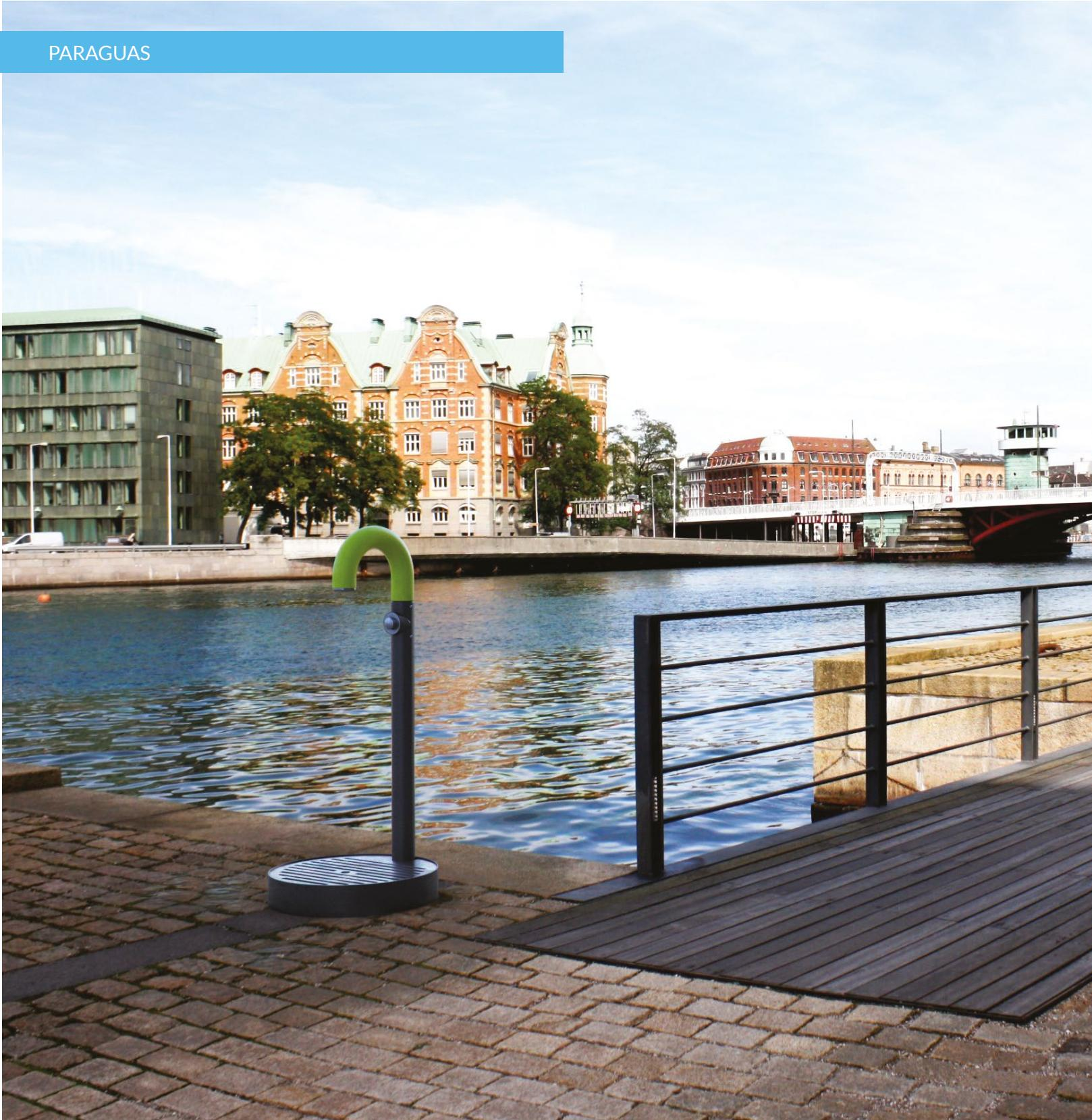
Drinking fountain composed of a steel tube structure, a chrome-plated brass tap with push button provided with a return spring and a circular tank. The latter is equipped with a drainage pipe with an overflow system and a removable drain for cleaning purposes.
