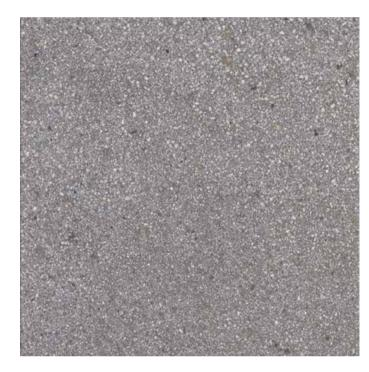
Features: to produce grey concrete, portland cement is used with inert materials from local quarries.
